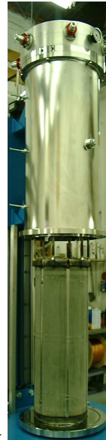
Large Tungsten-Mesh Element for an OXY-GON Bottom Loading Furnace
