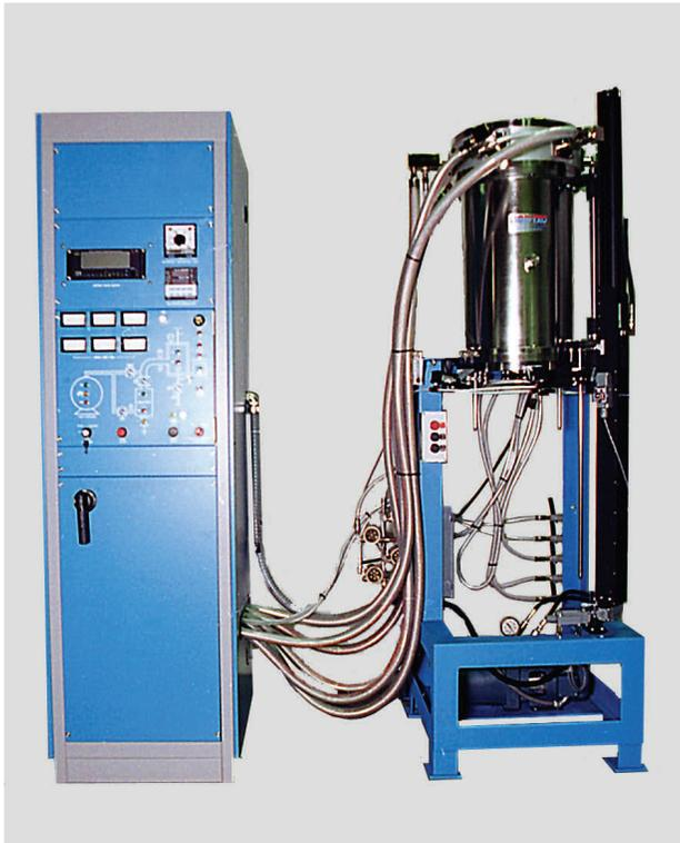
**The furnace can be rated up to a maximum operating temperature of 2500°C (4532°F) and will operate in vacuum, inert atmospheres, Nitrogen and wet or dry Hydrogen.**
